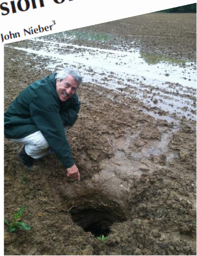
Figure 7. Sediment entering a soil pipe by interception of runoff by a pipe collapse feature in Goodwin Creek Experimental Watershed (GCEW).
